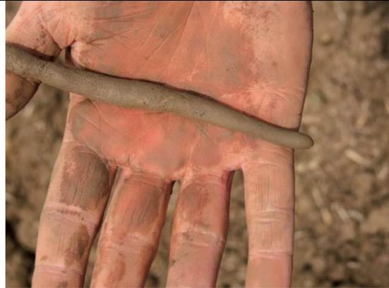
Fig-II Course grained soil roll with thread crumbles diameter 3mm
