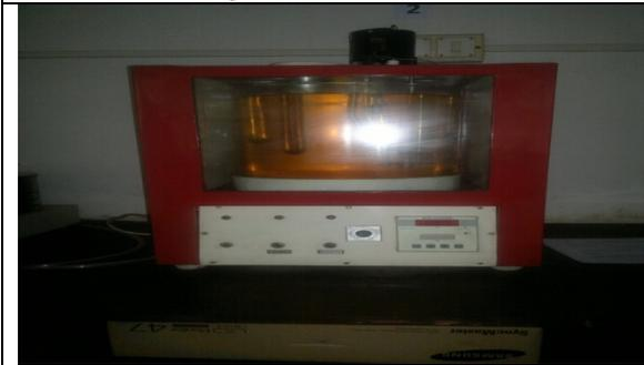
Fig.3. Kinematic viscometer bath apparatus
