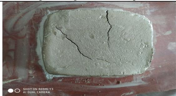
Fig 4. CDA (burnt), soil, white gypsum in (1:1:2) and(2:1:5)
