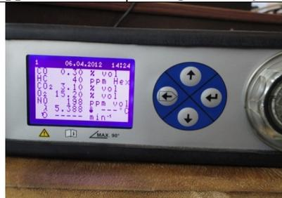
Fig 7. Exhaust gas analyser
