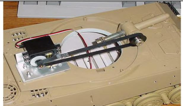
Figure.4 - Servo controlling swivel of a tank turret (RC tankcombat.com, 2007)
