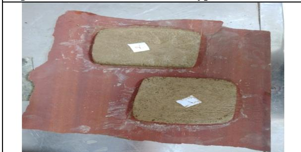
Fig 3. (1:1:2) and (2:1:1) gives a proper appearance but strength is very less
