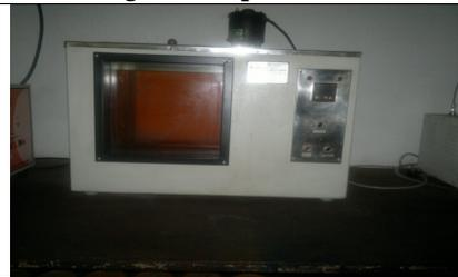
Fig.6. Density bath with hydrometer apparatus
