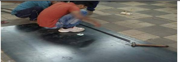
**Fig.2. MARKING OF MILD STEEL PLATE FOR PREPARATION OF COLLECTOR BASE**
