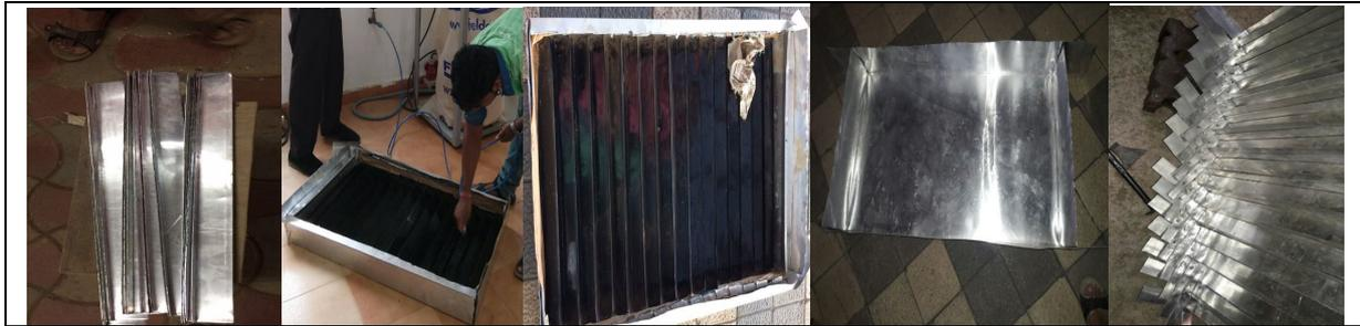
Fig.3. Making Collector Cover and Riveting the stairs
